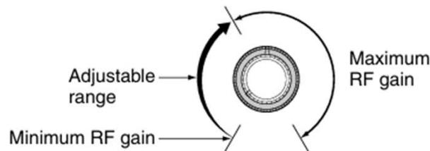
While rotating the RF gain control, a faint noise may be heard. This comes from the **DSP** unit and does not indicate an equipment malfunction.
