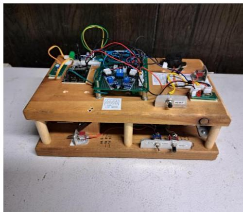
Once everything is working properly on the prototype, you can transition to a final design in an enclosure. Be careful of wire routing and signal types when transitioning to ensure you don't get signal crosstalk. In the final design it is always good to make sure you have bypass capacitors to reduce switching noise – especially in digital projects with high clock rates.
