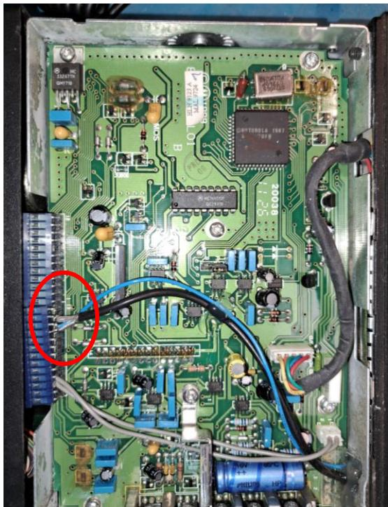
The figure above shows the modification to J8 of the Maxtrac. Pin 12 is the microphone audio input, pin 11 is the
