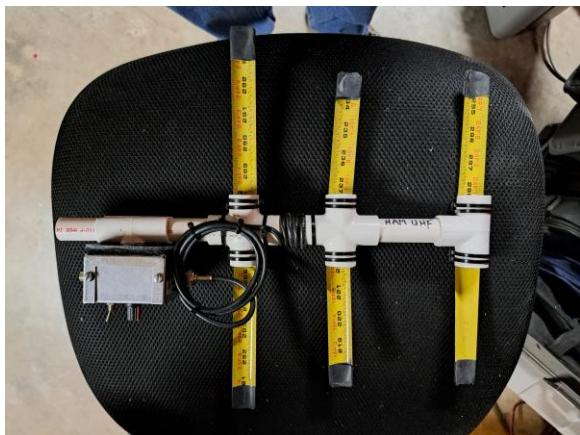
The above photo is one which I have built with an offset attenuator attached to the handle with the equipment shuttle described in a previous newsletter. The VHF beam we built as a team is shown below.
