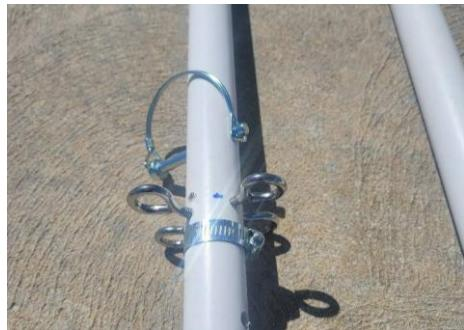
These holes don't need to be in a particular location, so give yourself some room. Also, with this configuration you could move the inner pipe 2"-3" on both sides of the hose clamp and use the outer pipe as a guide to give you height adjustment. I added a piece of painter's tape to the joint to hold the pieces in place before drilling the holes. If you want, you can also add painter's tape at each joint (around the 1.00" diameter pipes) to create a tighter fit between the inner and outer pipes.
