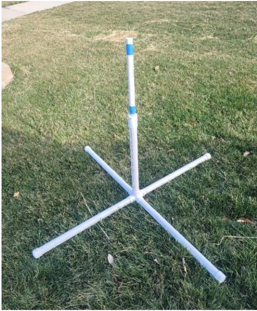
Slide a 1.00" diameter PVC pipe down through the 24" long 1.5" diameter PVC pipe until it protrudes out the other end. Take the 1" blue painter's tape and wrap it around the pipe so it just fits back into the end of the 1.50" PVC pipe. This will keep the lowest section of the 1.00" pipe stable (won't wobble around inside the 1.5" diameter pipe). Slide the 1" pipe so 28" extends above the reducer. Cut off excess pipe.
