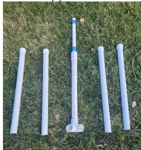
Cut all the 1.00" and 1.25" diameter PVC pipes in half, resulting in (6) 1.00" diameter and (6) 1.25" diameter PVC pipes.
