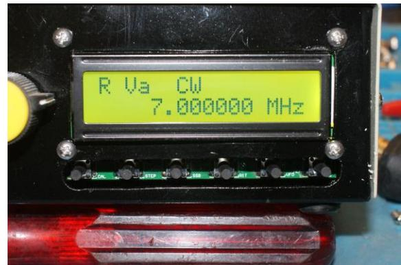
The finished product has a decent look to it and it may well end up in a stacked design with a buffer amp, modulator and power amp to make a QRP set.
