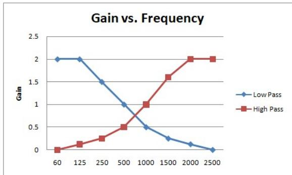
The plot above is as close as I could get with my audio generator and oscilloscope. It gives the general idea. The brown/red plot is with the HI pot at max and the LO pot at minimum and the blue plot is vice-versa with the LO pot at max and the HI pot at min.
