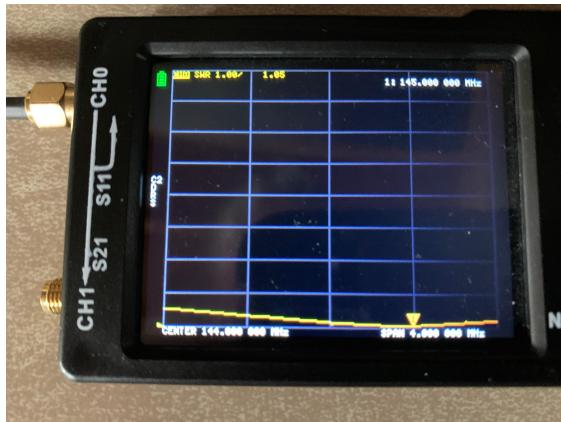
The magnetic mount antenna and the NanoVNA in this photo are sitting on a steel desk. When they were sitting on a wooden table with wheels the SWR was higher, about 1.5 to 1. The steel desk is in my basement is a better ground plane for the mag mount antenna since it has a copper ground strip sitting on it that is connected to a copper water pipe.
