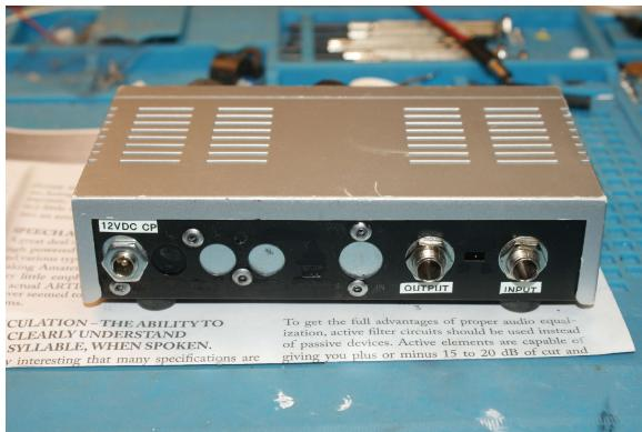
Anyway, the circuit has an overall gain of about two or 6 dB with high and low pass/attenuation where the low cutoff is around 500 Hz and the upper cutoff is around 1 kHz to allow the intelligibility part of the voice spectrum while dampening the lower frequencies (500 Hz and down) that make the voice sound muddy and difficult to copy. The attenuation is variable to allow flexibility in the "tone" from the microphone through the equalizer.
