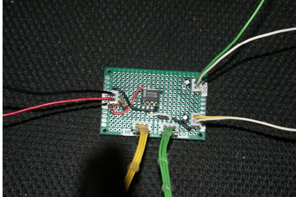
Most of the components are capacitors and resistors which I mounted to the potentiometers for convenience sake. The HI potentiometer has the passive components for the high pass part of the circuit and the LO potentiometer conversely, has the components for the low pass part.
