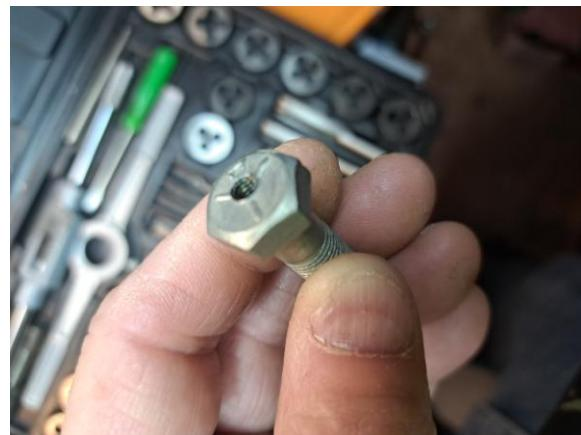
Use oil on the tap as well – note the threads in the bolt head hole.
