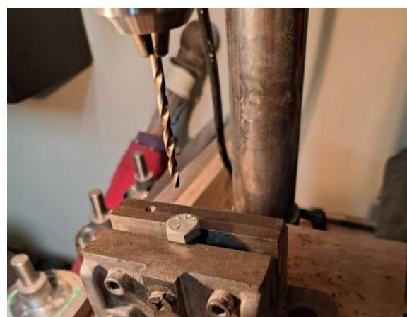
Use liberal amounts of oil while drilling to keep the bit cutting, not wearing out.
