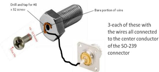
The drilling was done on my drill press using a 9/64 bit with a #8-32 tap to thread the hole.
