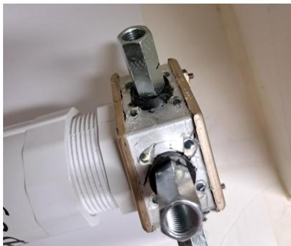
I drilled a hole in the center of the top of a 3/8" x 24 bolt (½ to ¾ inch long). The hole should be deep enough to accommodate an #8-32 by ½ inch screw. Then thread the hole for the said screw. This has to be done on the three 3/8" x 24 bolts that are on the insulated coupling nuts. The #8 x 32 screws are for attaching a wire from the nut to the center conductor of the SO-239 connector.
