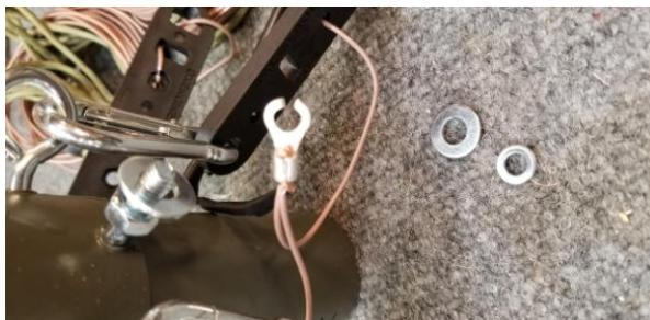
The ring terminals are then secured to the posts on each side of the cap; Since the posts are in the same cap without insulation, I packed some leftover foam from a pelican case to prevent arcing or shorting.
