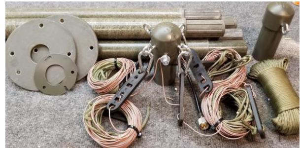
A different configuration substitutes 450ohm ladder line and a remote tuner (tuner installed at the base of the antenna). The alternate configuration may yield better performance, but requires a remote tuner and ladder line in addition to the pieces listed above – main difference for the build using the ladder line is to skip the coax pigtail and connect the ladder line directly to the cap, one lead on each post.
