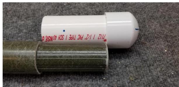
I measured and cut a piece of the 1 ½ in pipe to fit over the pole and left enough clearance over the top of the fiberglass so that once an end cap was added, the entirety of end cap area would clear the fiberglass pole – this is important because we are going to be drilling holes and screwing things into the end cap and we do not want to damage the fiberglass. The next step is to mount anchor points into the end cap for the antenna wires, 4 supports in total; I chose #6 ring bolts.
