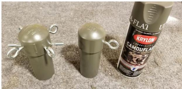
The four eye bolts will soon hold the wires, and the two posts on each side are “hanger bolts”, coarse threaded on one end and machine threaded on the other end; Those will be used to connect the ends of the wires to the feed point harness via ring terminals. The wire dimensions are as follows:
