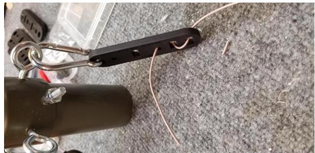
For the feed point, I took a short piece of RG8x with a PL-259 on one end and the other end was stripped back, creating two leads; One from the center conductor and one from the shield. The antenna wire is 14ga stranded copper. I stripped the antenna wires back (brown wire in the picture above) and paired them as follows:
