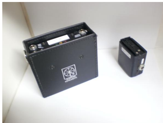
Redesigned Quantum Battery Pack (now 12 V Li-Ion) with the Battery Adapter Pack
