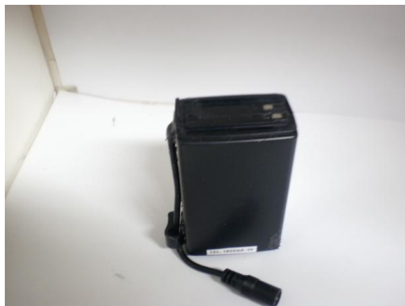
NiMH 1500 mA-Hr Battery Pack Converted to 1800 mA-Hr Lithium-Ion Pack
