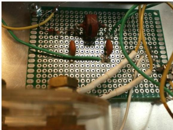
The beauty of this project is in its simplicity. We all remember the old crystal radio receivers we built as a Science Fair project or just for fun. This is very similar. The germanium crystal diode works as an envelope detector, the two capacitors and inductor as a filter and the resistors are for scaling for the meter.
