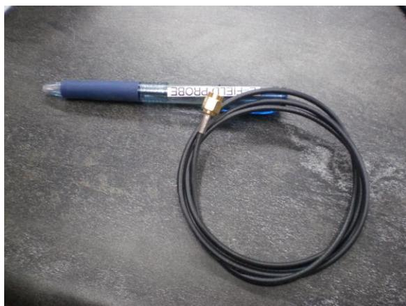
The bare part of the coax center conductor essentially works as a small antenna.
