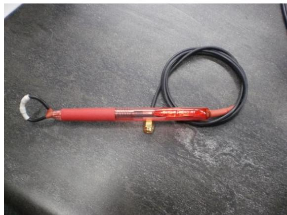
Since radio waves have both a magnetic and electric field component. Either probe should work. The E-field probe is easier to get into tight areas. I put the E-field probe in the blue pen body and the H-field probe in the red pen body. Both work great and I used both to troubleshoot the UBITX V4.3. If you have a spectrum analyzer, I hope you find this article useful. There are a few other things I want to do with the
